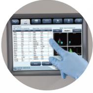
SPU with touch screen is used for sample processing, including QC, calibration & maintenance. DMU by PC is used for data management only. the PC software allows easier operation and wider application.
