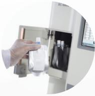
Replacement of the fluorescent reagents in BC-6800 is very convenient as the reagent compartment is located on the left front of the analyzer.
