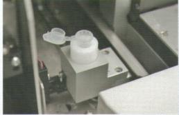
The SC-120 can make smear from capillary samples as it requires only 40µL blood.
