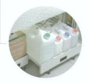
All reagents as well as the pneumatic unit could be set in the trolley below respective BC-6800 or SC-120. In this manner, the reagents and pneumatic unit could be well organized permitting easy reagent replacement.
